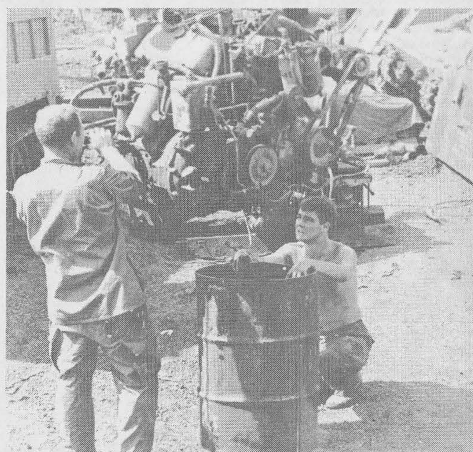
The engine of an ACAV is suspended as troopers from K Troop perform maintenance during a short standdown at Quan Loi.
